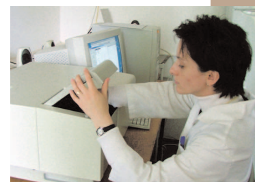
Photoluminescence measurements (Spectrofluorimeter Wave, JASKO FP-6500)
