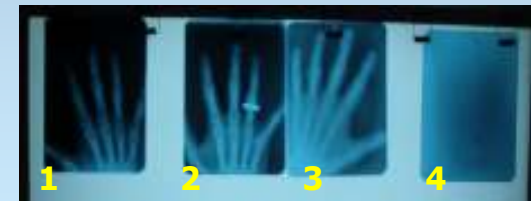
Radiographies performed using: EIRX (1,2), standard screen from the market (3) and no screen (4)
